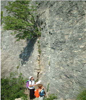
Index analysis RMR in wall used for free climbing (Pietra di Bismantova, Emilia Romagna)
